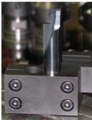
▲ Custom cutting toolholders can be matched to the machining requirements, making very complex form tool machining a practical option to be used as the Hydromat or single-spindle CNC turning centers.
